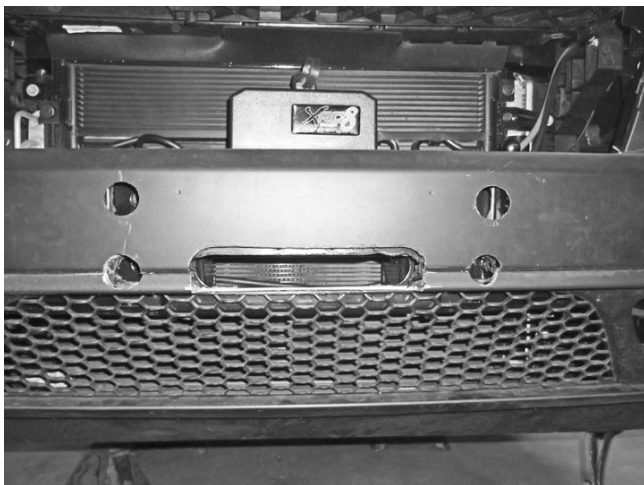
< Photo at left shows the oval and spacer tube mounting holes drilled and cut.
